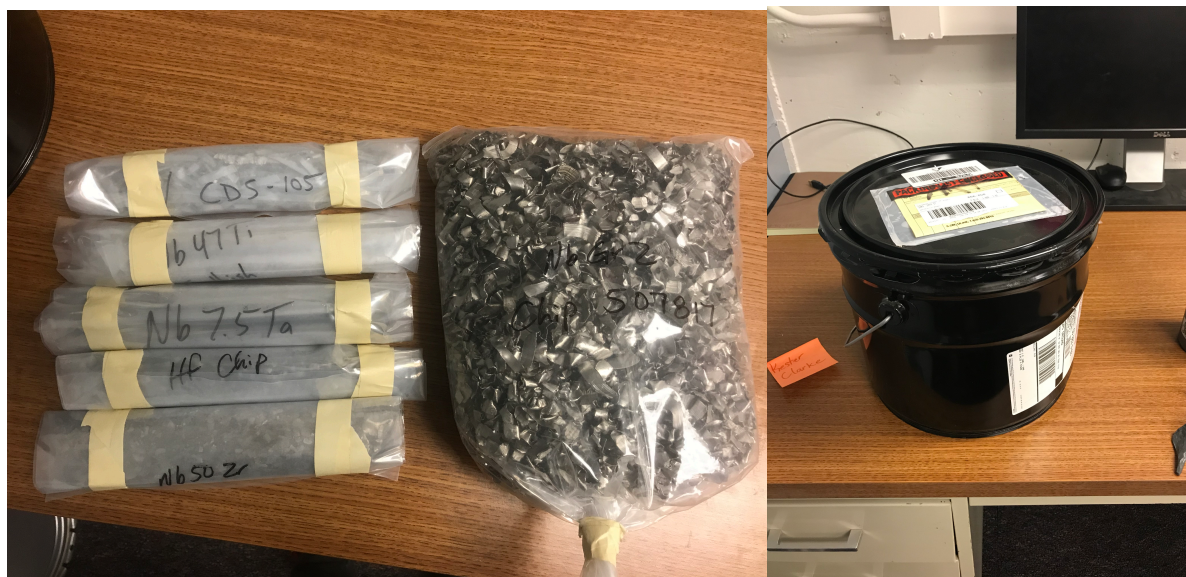
Figure 60.1: The above picture shows the materials recently acquired for binary alloy manufacturing, supplied by ATI Materials. Contents include, Nb chips, Hf chips, V chips, Nb50Zr chips, Nb47Ti rod, and Nb7.5Ta rod. More materials are expected to arrive in the near future. Also pictured is the bucket they arrived in for scale.
