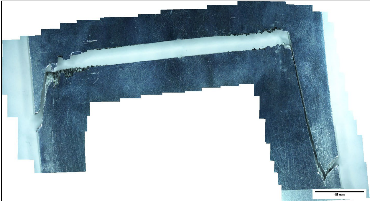
Figure 48.4: Image mosaic from stereomicrographs along the full fracture edge of plate MH-LS-01.
