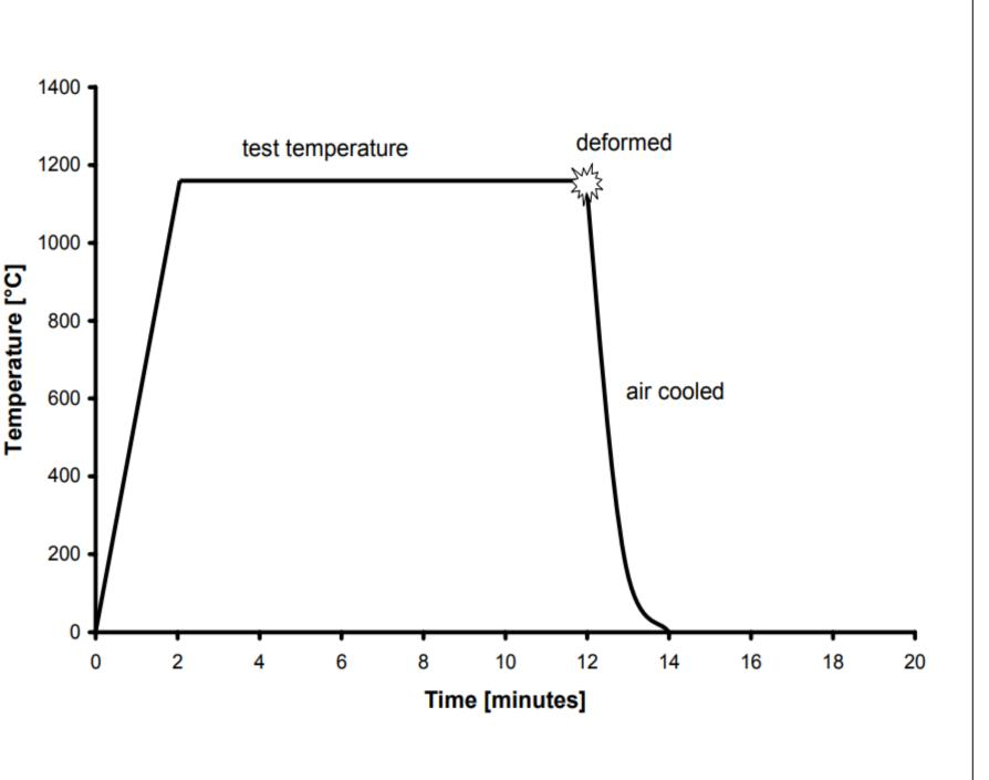
Compositionally graded copper/nickel additive samples are being prepared to explore spectrum of hot shortness behavior as a function of copper, nickel composition.
