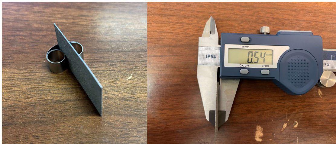
Figure 52.5: Thin plate that is about two melt pools in width. The plate is then modeled in Abaqus and the predicted microstructure from the GV map is then compared to the microstructure observed in this plate.
