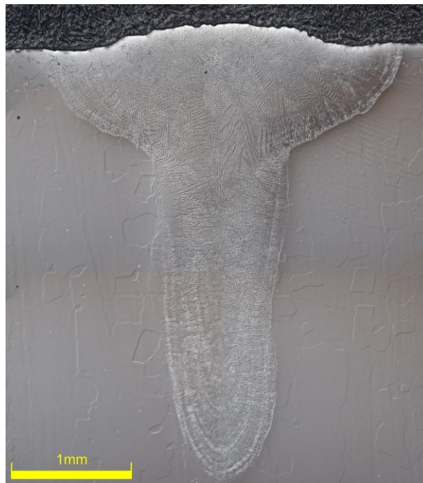
Figure 36H-L.4: An LOM image of an etched laser track melt cross section in Nb-47Ti showing significant keyholing, rather than the more desirable conduction-mode melting. Sample was etched with Kroll’s Reagent.
