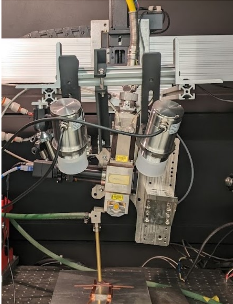
Figure 36H-L.2: Interior of laser welding cabinet with Nb-47Ti sample positioned immediately below Argon delivery tube and collimating optics and fiber optic cable above.
