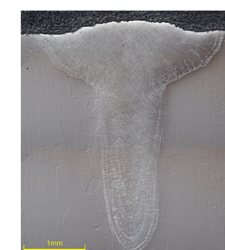
Nb-47Ti weld cross-section showing keyholing
