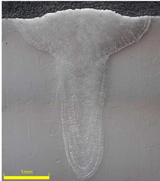
Significant keyholing in Nb-47Ti laser track melt using published L-DED parameters
