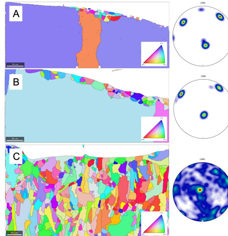
Inverse Pole Figure (IPF) map and Orientation Distribution Function (ODF) near the end of a raster of Inconel 718 under various conditions.
