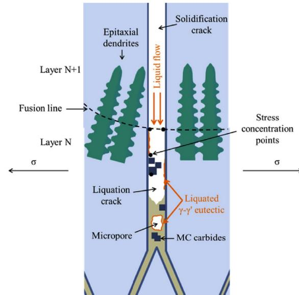
Schematic diagram of hot cracking.
