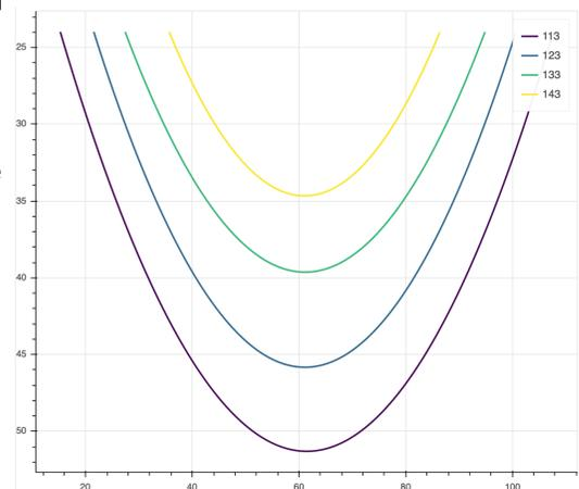
Relative pixel location of solid/liquid interface at various frames for Inconel 738 at 108 Watts.
