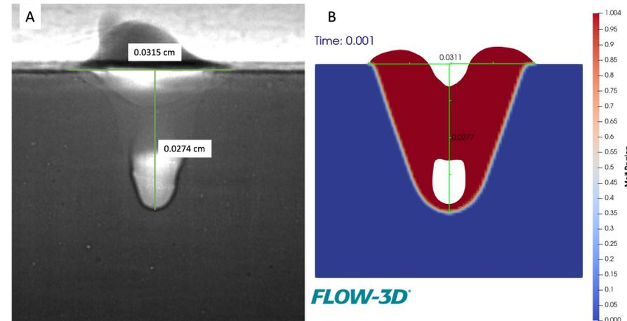
Dimensional comparison of synchrotron x-ray radiograph and simulated spot melt.
