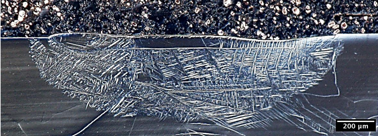
Figure 36A.12: Stress induced \alpha'' in an etched Ti-10-2-3 AM sample melted at the Advanced Photon Source. Parent \beta -Ti grains are not obvious in the melt pool region and cannot be reliably inferred from the orientation of the martensite plates.
