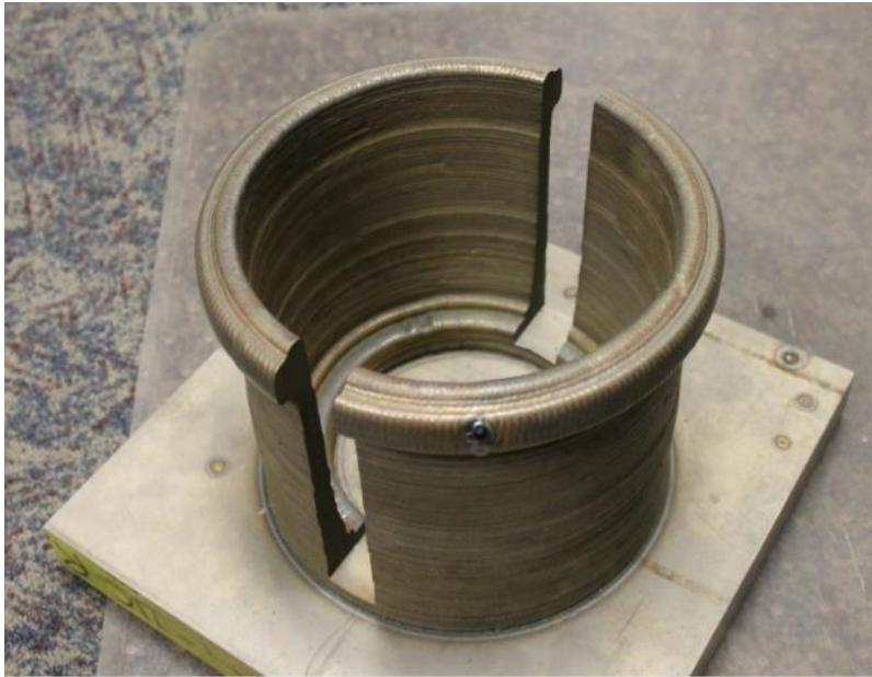
Figure 36A.1: Full build volume WAAM Ti-6Al-4V samples were extracted from for characterization (courtesy of SNL). Samples were extracted from the two cut out sections via wire EDM.
