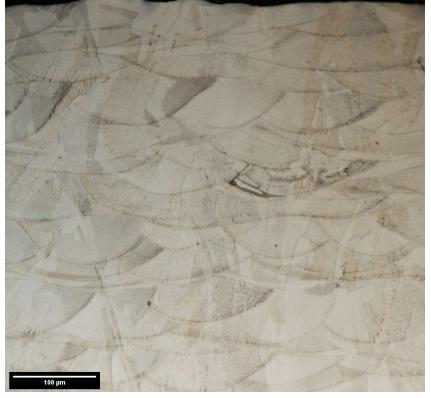
Discrepancies between Rosenthal model predictions and experiments are likely due to a combination of sectioning effects and the limiting assumptions in the model.
