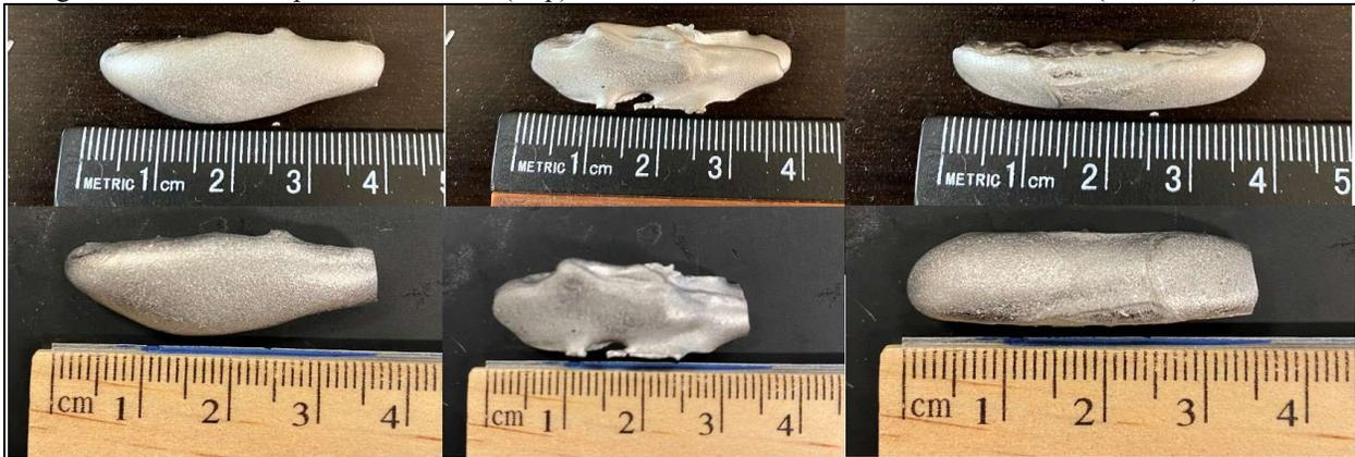
Figure 46.3: Ta<sub>4</sub>Ti<sub>3</sub>Cr specimens, as-cast (Top) and after HIP at 1400 °C, 30 ksi for 3 hours (Bottom).
