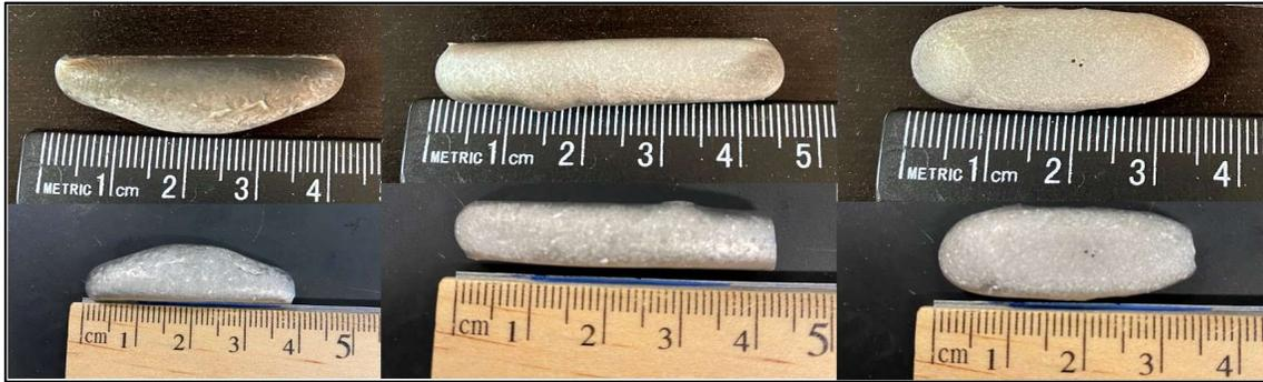
Figure 46.1: TaTiCr specimens, as-cast (Top) and after HIP at 1400 °C, 30 ksi for 3 hours (Bottom).
