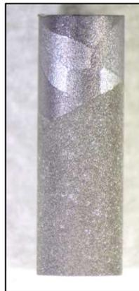
Figure 46.5: Compression specimen with unmixed tantalum
