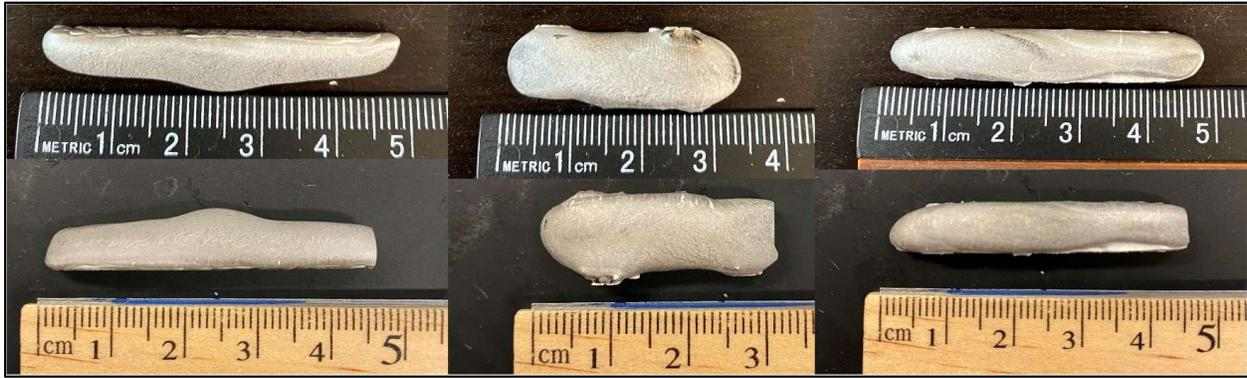
Figure 46.4:  $Ta_4TiCr_3$  specimens, as-cast (Top) and after HIP at 1400 °C, 30 ksi for 3 hours (Bottom).
