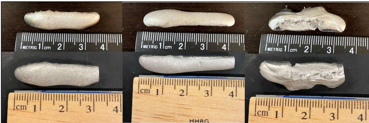
Figure 46.2: Ta<sub>2</sub>TiCr specimens, as-cast (Top) and after HIP at 1400 °C, 30 ksi for 3 hours (Bottom).
