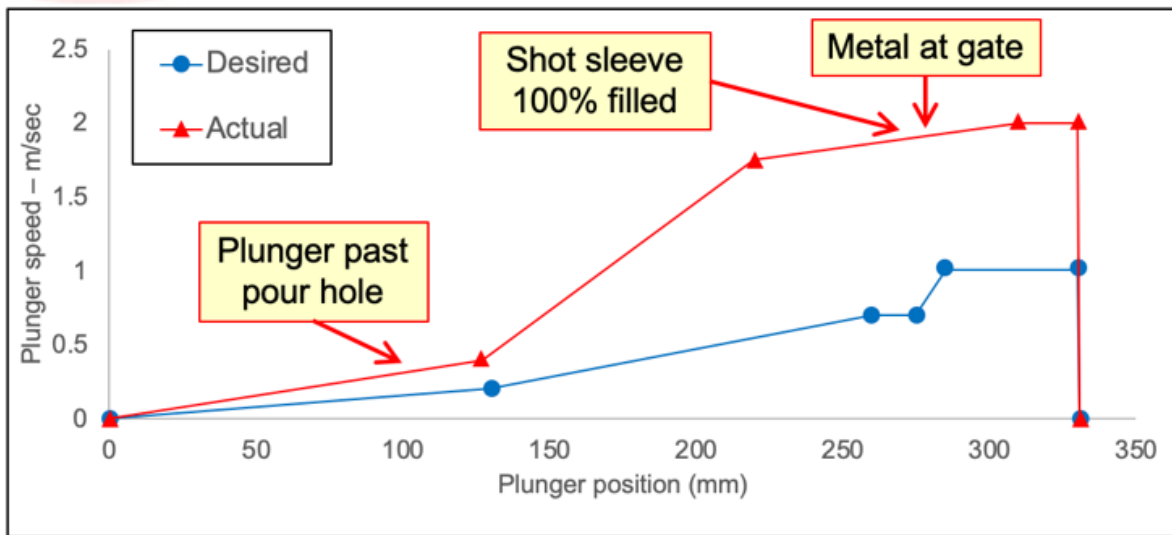
Figure 37.2: Differences in shot profiles from the desired to the profile actually used during the test.
