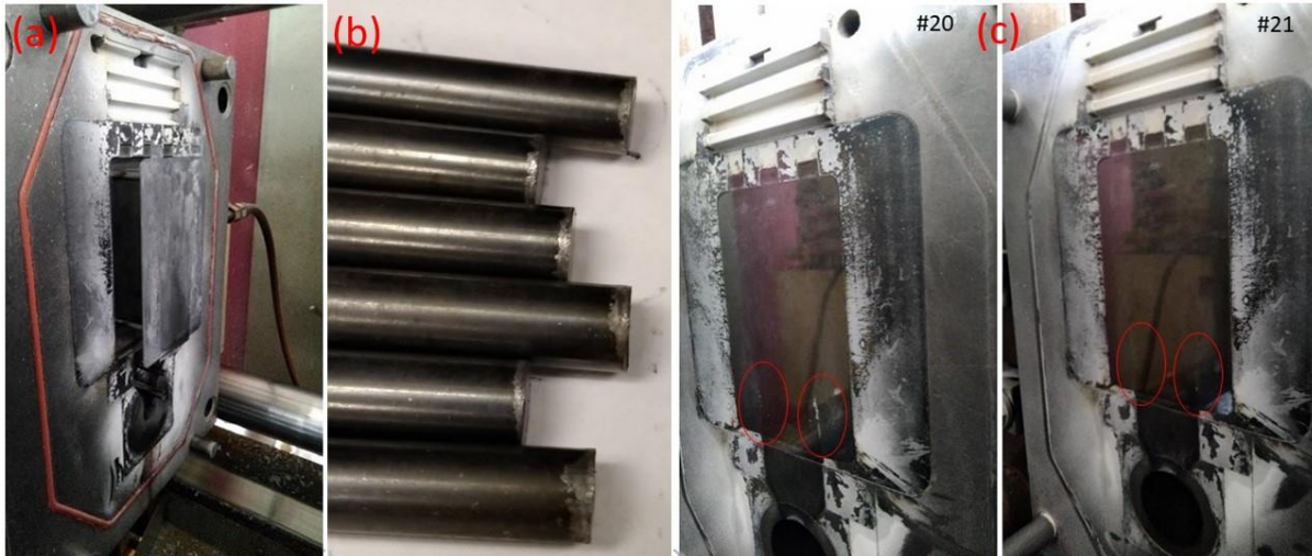
Figure 37.3: Lube-free casting trial using die #1 where (a) ejector side showing the casting stuck to the tip of the ejector pins, (b) side of tip of the core pins with aluminum adhered, and (c) intermittent aluminum build-up at the coated die surface appearing at casting #20 and disappearing at casting #21.
