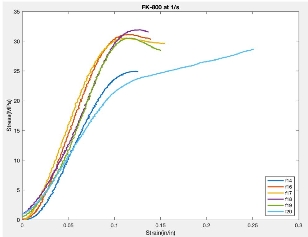
Figure 44.3: Stress v. Strain plots from compression testing of geometrically identical FK-800 samples (cylindrical, 0.25” high, 0.5” diameter)
