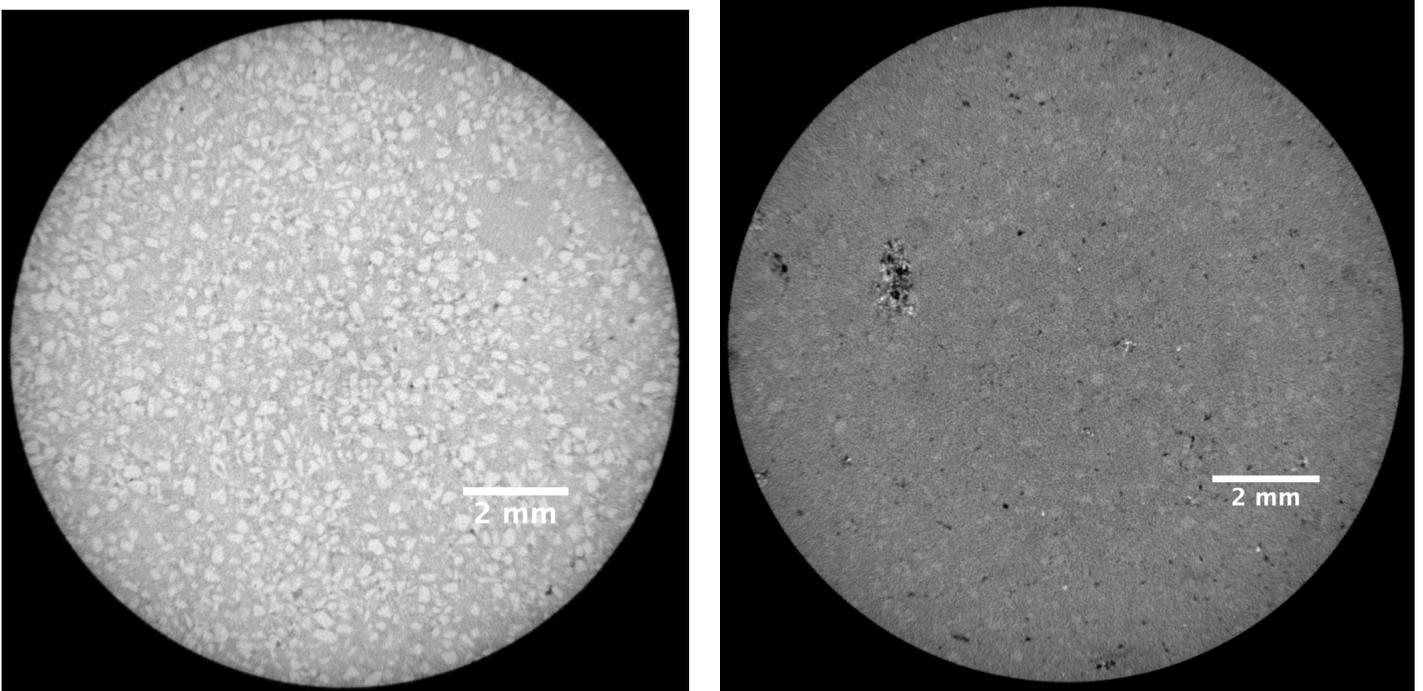
Figure 44.5: Cross section through a CT image of pristine MHE (left) and recycled MHE (right)
