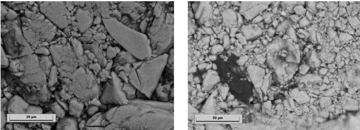
Figure 44.4: SEM imaging of pristine MHE (left) and recycled MHE (right)
