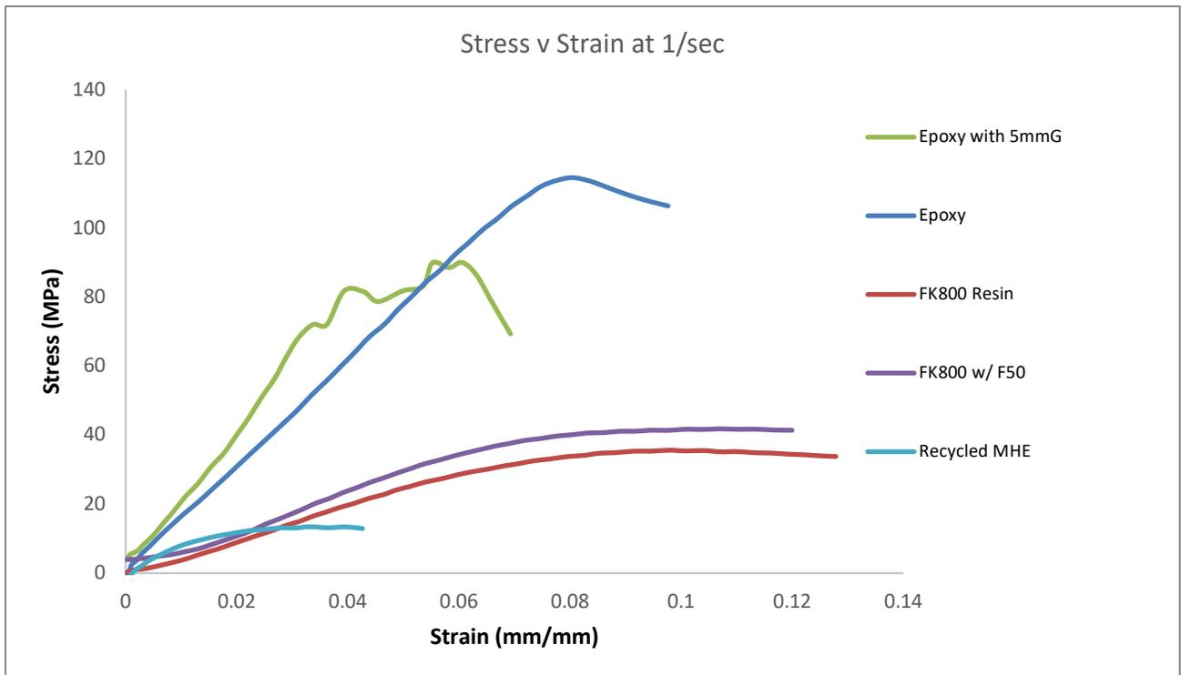
Figure 44.2: Stress v. Strain plots from compression testing of preliminary mock HE materials and recycled MHE
