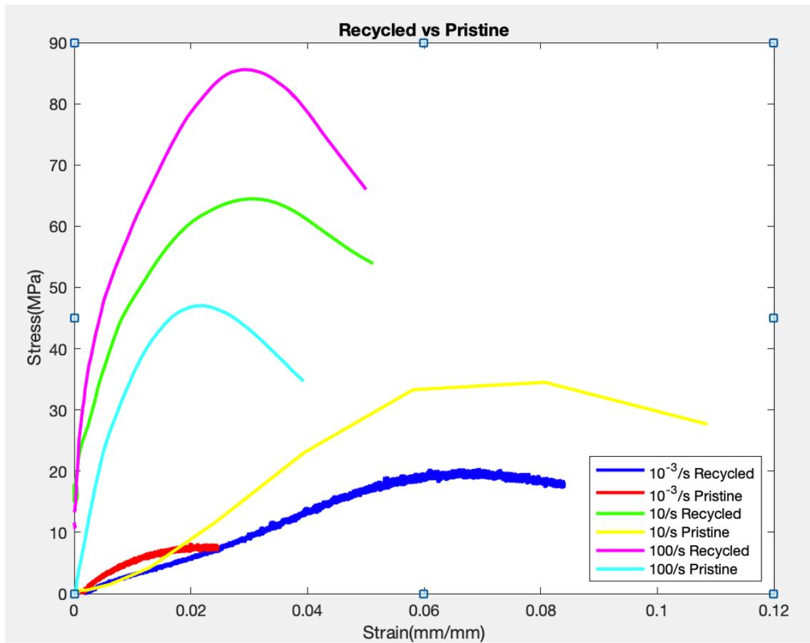
Figure 44.1: Stress v. Strain plots from compression testing of pristine LANL MHE and recycled MHE
