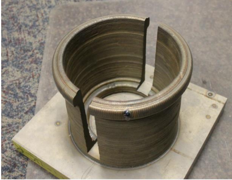
Figure 36A.3: Full build volume WAAM Ti-6Al-4V samples were extracted for characterization (courtesy of SNL). Samples were extracted from the two cut out sections via wire EDM.
