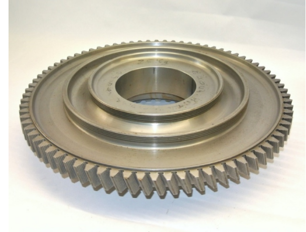
High pressure turbine disk Approximately 50cm diameter
