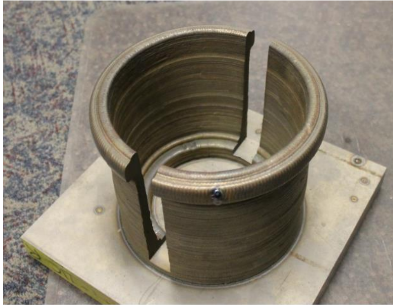
Figure 36.3: WAAM Ti-6Al-4V samples extracted for characterization (courtesy of SNL).
