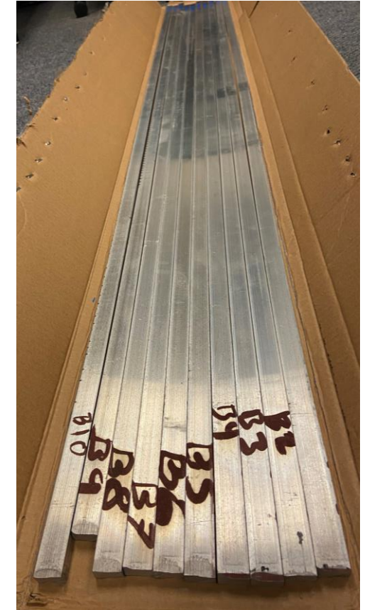
10 billets of experimental material, 2 of each alloy composition, with the cross-section geometry of 1/2" x 7/8"
