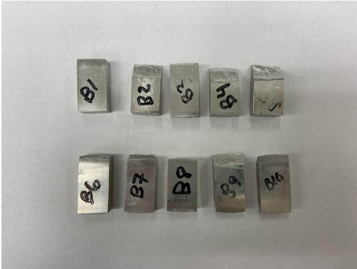
Rolled experimental ZK60 samples. Initial dimensions: 1/2 " x 7/8 " x 1/4 "
