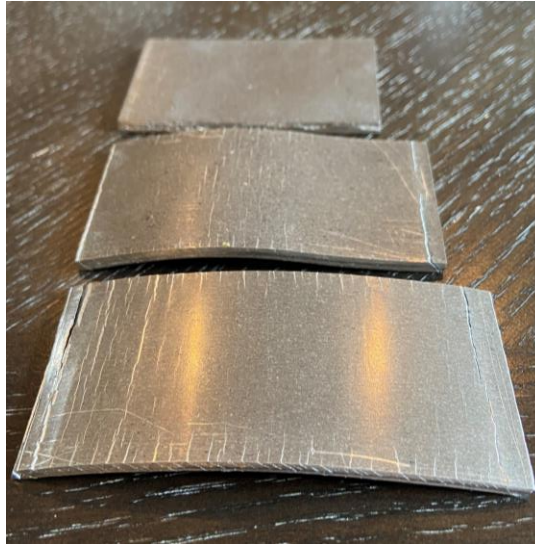
Figure 39.5: Rolled AZ31. From top to bottom: 0% reduction in thickness (not rolled), 15% reduction in thickness, and 18% reduction in thickness. Initial geometry of these samples before rolling is 3" x 1.5" x 0.125".
