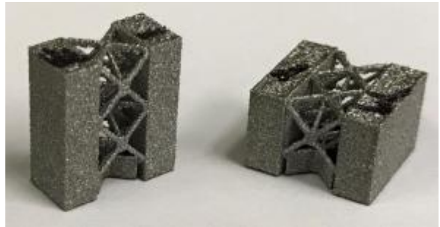
Ti-5553 Lattices from LLNL; ~11.4 mm and ~9.5 mm largest dimension
