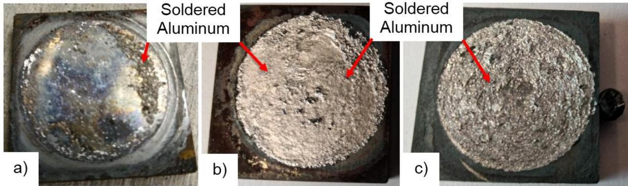
Figure 37.4: Surface condition of the H13 steel substrates (after Al casting removal) ground to 600 mesh after holding times at 700 °C of a) 15 minutes, b) 1 h, and c) 4 h.
