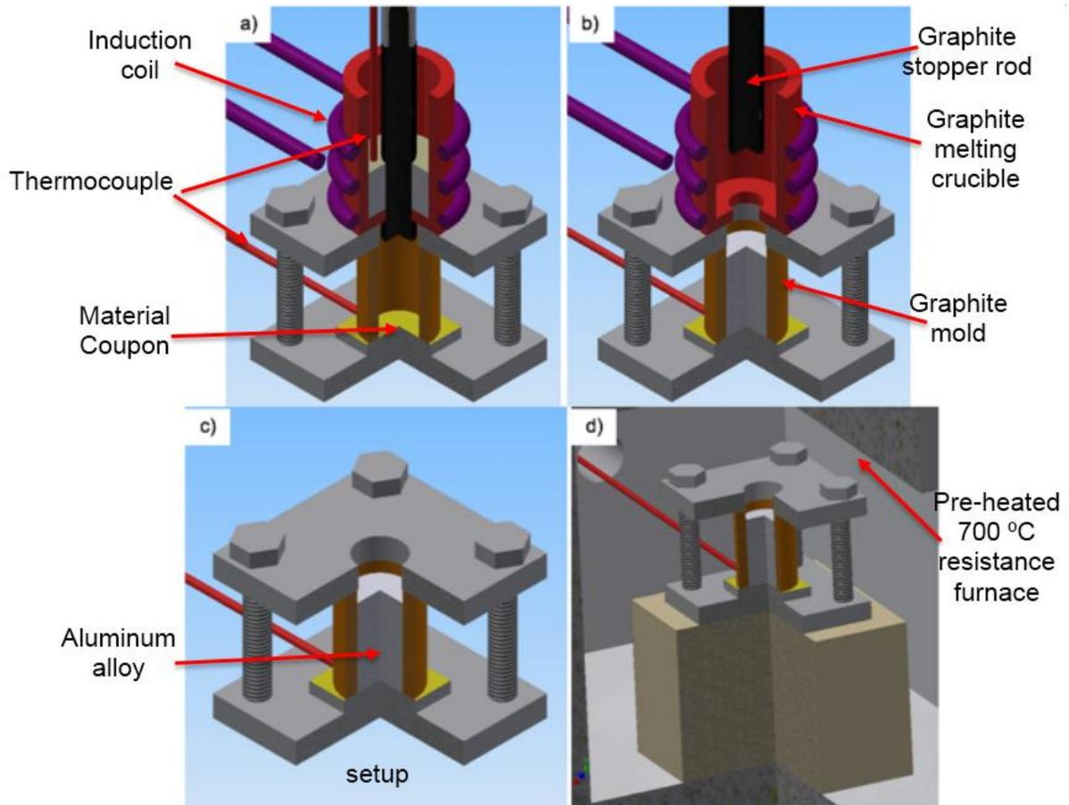
Figure 37.1: Improved test apparatus: a) induction melting of aluminum alloy, b) bottom pouring by lifting the stopper rod, c) removing the lower portion of the apparatus from the induction melter, and d) placing the apparatus inside a resistance furnace preheated to 700 °C.
