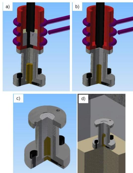
Figure 37.7: Schematic of new H13 mold testing a rod material coupon: a) induction melting of Al alloy; b) bottom pouring by lifting the stopper rod; c) removing the lower portion of the apparatus and d) placing inside the resistance furnace preheated at 700 °C.
