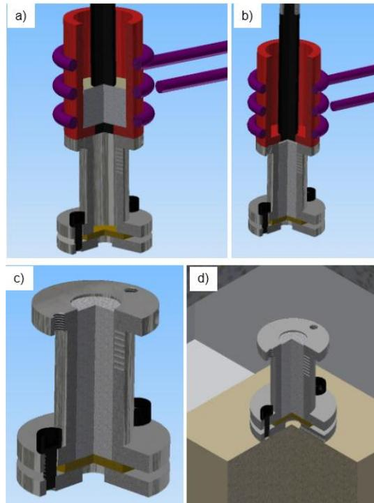
Figure 37.6: Schematic of new H13 mold set up for testing a flat material coupon: a) induction melting of Al alloy; b) bottom pouring by lifting the stopper rod; c) removing the lower portion of the apparatus and d) placing inside the resistance furnace preheated at 700 °C.
