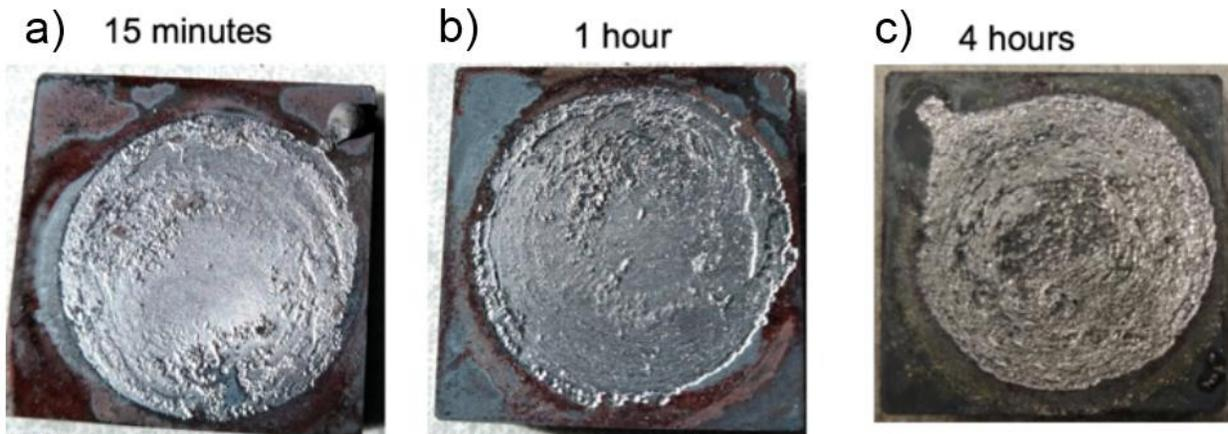
Figure 37.5: Surface condition of the H13 steel substrates (after Al casting removal) polished with 1  $\mu\text{m}$  after holding times at 700 °C of a) 15 minutes, b) 1 h, and c) 4 h.
