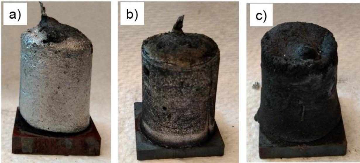
Figure 37.3: Al castings on H13 steel substrates ground to 120 mesh after holding times at 700 °C of a) 15 minutes, b) 1 h, and c) 4 h.
