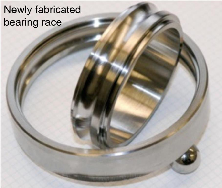
Water quenched and machined bearing (unused)
