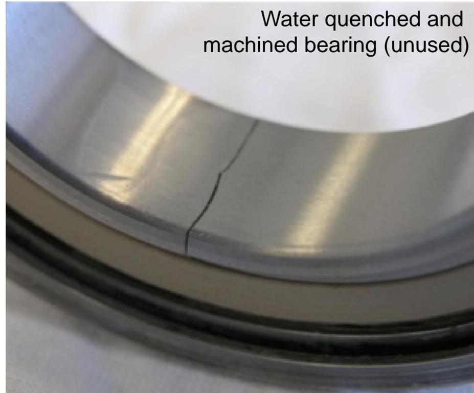
Residual stresses due to large undercooling (water quench)
