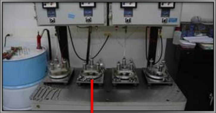
Spring loaded test head
