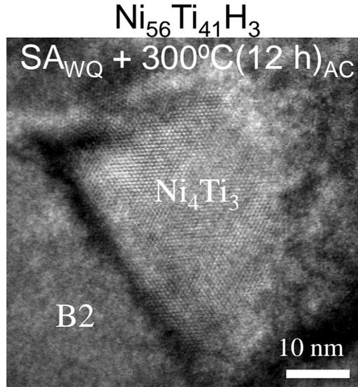
← Slows  $Ni_4Ti_3$  kinetics (NiTiHf retains high hardness with air cooling)
