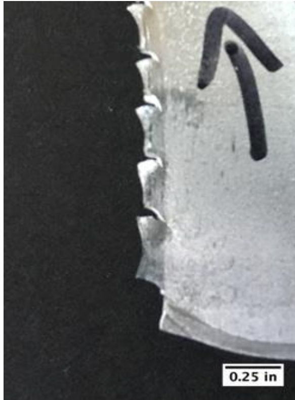
Material Overhang Al 2024 – 2 ARB cycles
