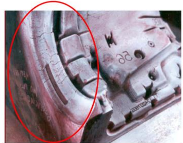
Heat checking of an H13 steel die
