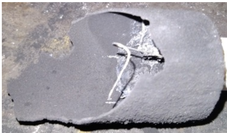
Figure 37.3: Photo of the graphite crucible after heating in air for several hours at 700 °C in a resistance furnace using the first iteration of the improved AAT.
