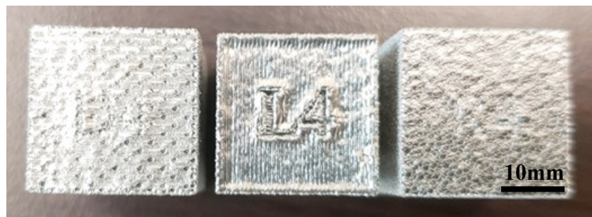
Figure 36.2: Photo of Ti-6Al-4V samples before sectioning. Note the different scan strategies as exhibited by the surface topography of the DeHoff scan strategy (left), the Linear Raster scan strategy (center), and Random (right).
