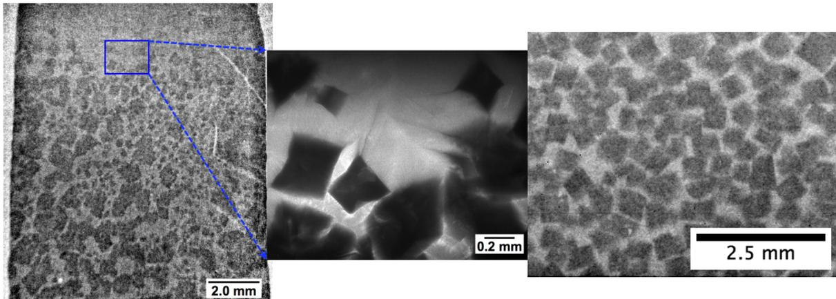
Figure 32.3: Proton (left) and synchrotron x-ray (center) radiographs showing the differences between the methods [32.1]. Synchrotron x-ray radiography exhibits a much higher spatial resolution, but proton radiography portrays a much larger field of view. Micro-focus laboratory x-ray radiograph (right) shows a good middle ground for spatial resolution and field of view [A.J. Clarke et al., unpublished research].
