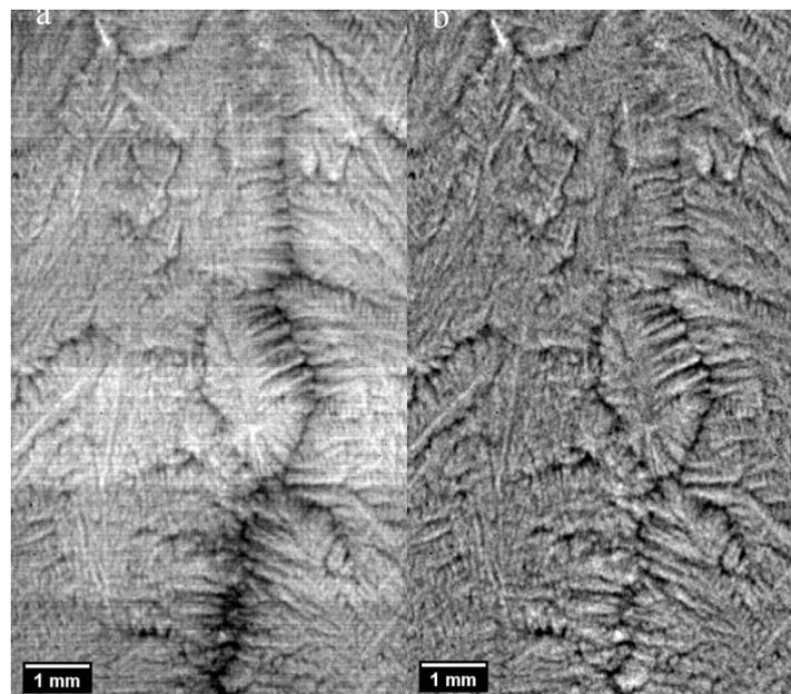
Figure 32.2: Further processing of the same frame of Al-Ag solidification shown in **Figure 32.1** by (a) trimming 10 pixels from each edge of the radiograph, allowing for better contrast in the solidification structure, and (b) performing fast Fourier transform filtering to remove horizontal and vertical banding artifacts.
