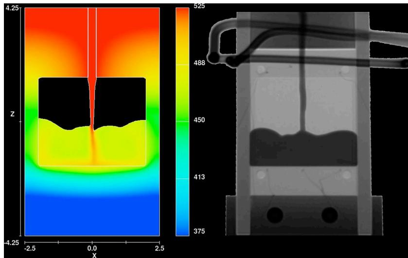
Figure 32.5: Casting model (left) informed by proton radiography of a Sn-Bi alloy (right). Further experiments and observation will bring the modeling closer to reality [A.J. Clarke et al., unpublished research].
