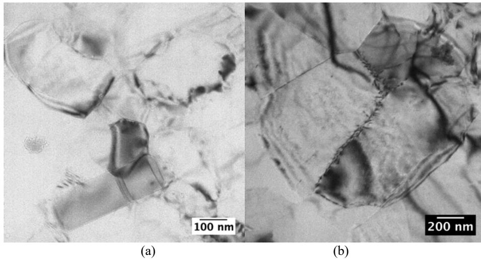
Figure 31.3. TEM micrographs showing submicron sized grains in (a) 8 cycle Al 1100 rolled at room temperature and (b) 5 cycle Al 5083 rolled at 250 °C.
