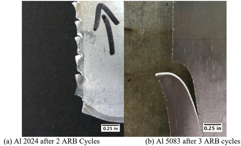
Figure 31.1: Edge cracking mainly caused by material overhang (a) and lateral spreading (b). In (a), the edge of underling material can be seen by faint line at the tip of all cracks. In (b), material overhang cracking was reduced by using copper binding wire to constrain sheets together; cracking instead resulted from tensile stress state that develops along the edge due to high lateral spreading. Rolling direction is bottom to top in both images.
