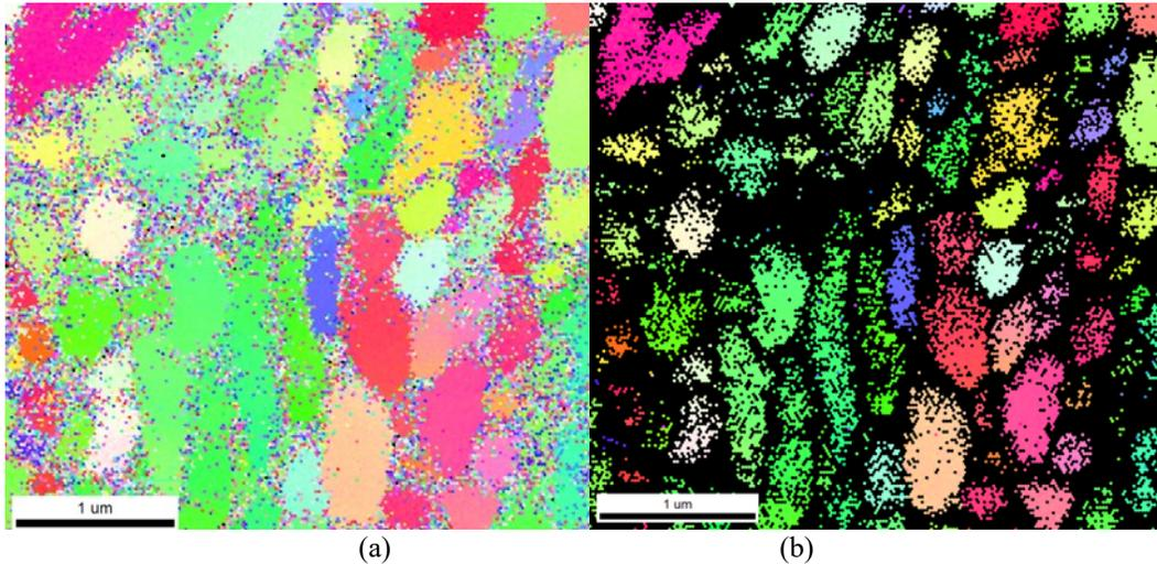
Figure 31.4. Inverse pole figure maps of 6 cycle Al 1100 rolled at room temperature. (a) shows raw data from EBSD scan, while (b) shows the same data filtered to remove points with a confidence index less than 0.1. It should be noted that grain interiors are indexed with high confidence.
