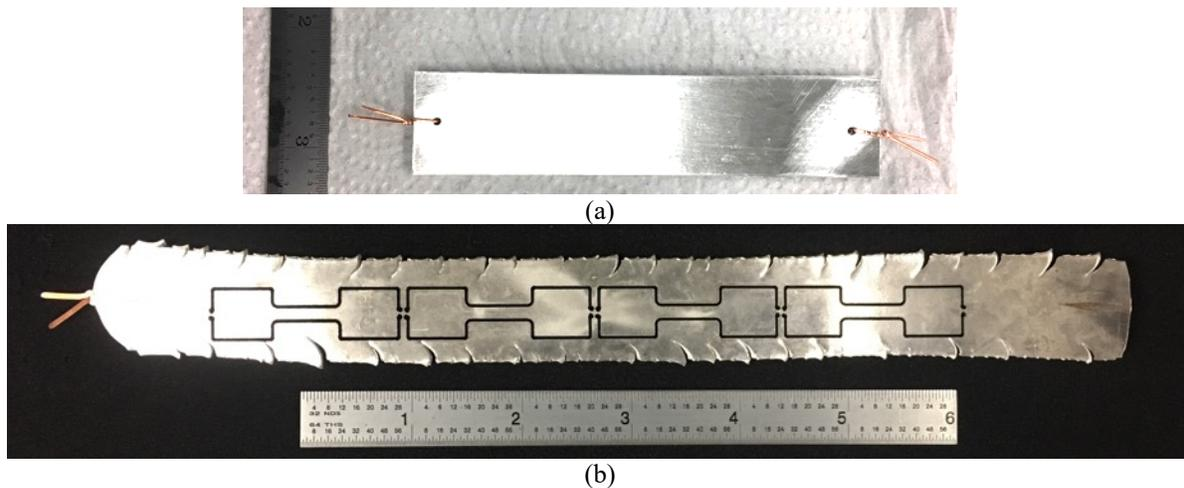
Figure 31.2: Al 5083 before (a) and after (b) 5th ARB cycle at 250 °C. The use of copper binding wire is shown in (a), which led to reduced material overhang cracking in (b). Scale bars are in inches.
