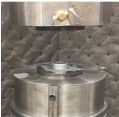
Figure 28.1: (a) Manufactured die sets with removable insert pairs. A different coating can be applied to each pair of inserts to test various surface treatments, and the inserts can be separately pre-heated in an air-furnace for elevated temperature ring-tests. (b) The die set inserted on the 100 kip MTS servohydraulic test frame at Mines. (c) Example rings tested to different reductions (increasing reductions for each column from left to right) and using different friction conditions (top row is unlubricated, middle row uses graphite spray, and bottom row uses MoS 2 grease), showing the difference in ring geometry as a function of reduction and lubrication conditions.
