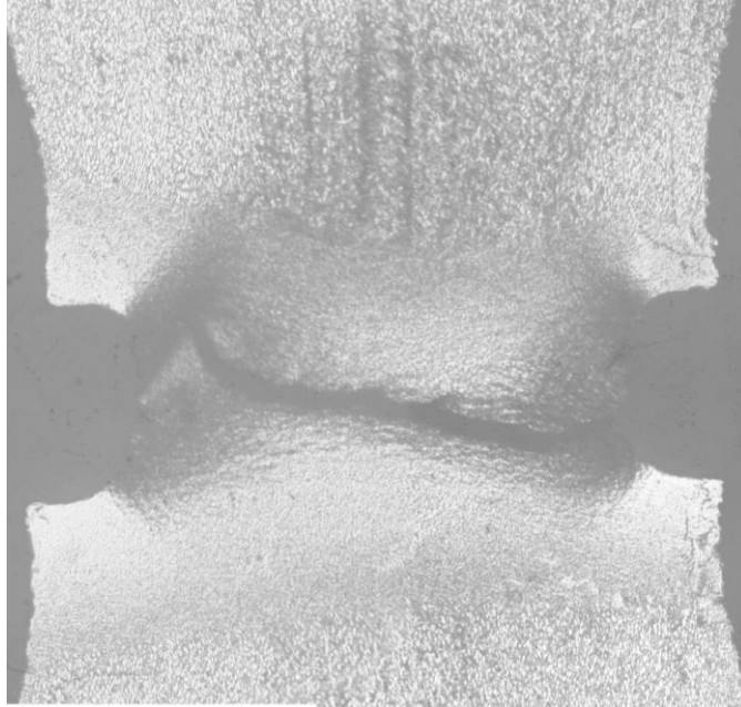
Fig. 7 WZ Tensile test specimens after test.
