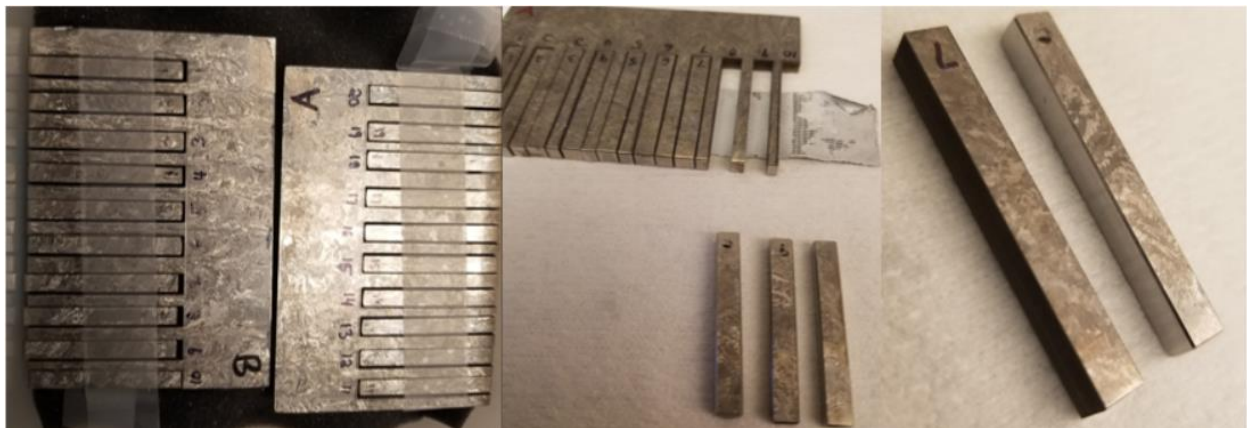
Fig. 11 Conventional fatigue beams sectioned via EDM, chamfered, polished and etched.
