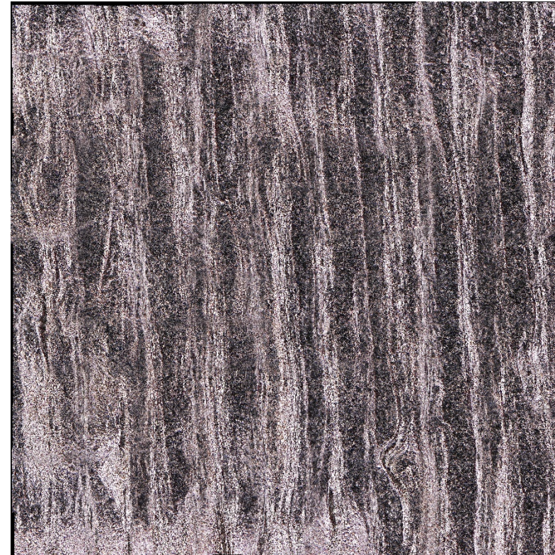
700X view of a Ti-6-4 sample surface
