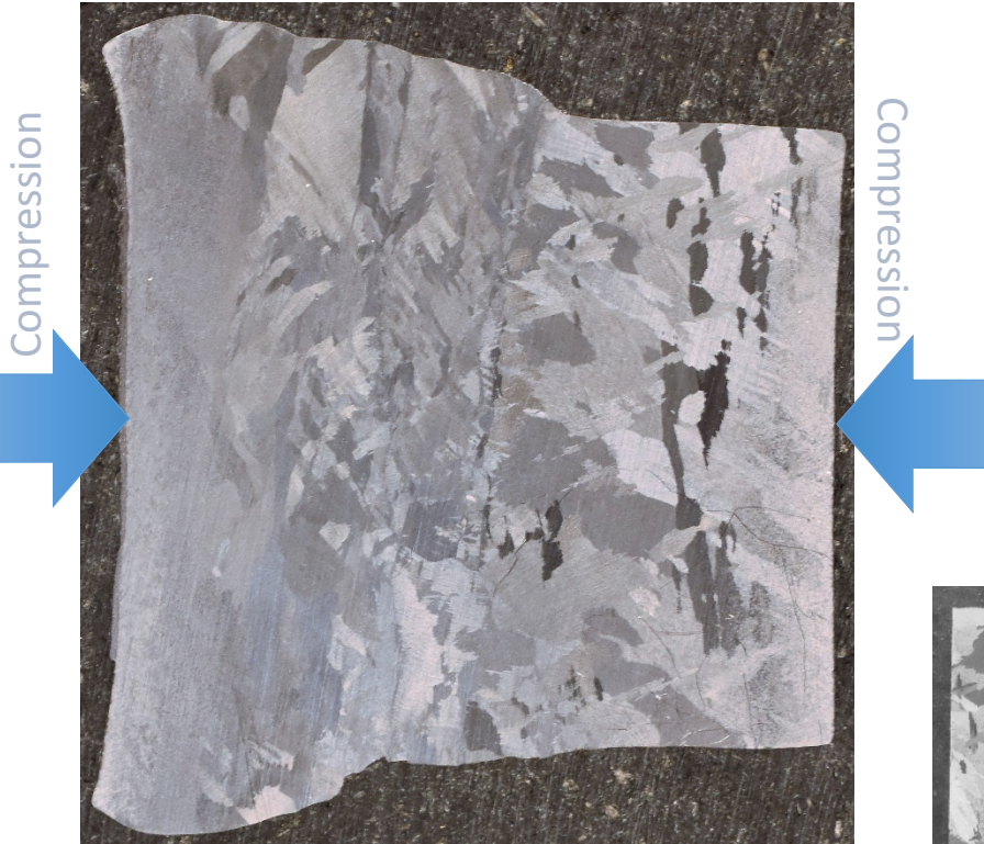
Sample machined from edge of billet, uniaxially compressed to 30% height reduction at 925^{\circ}C and macroetched
