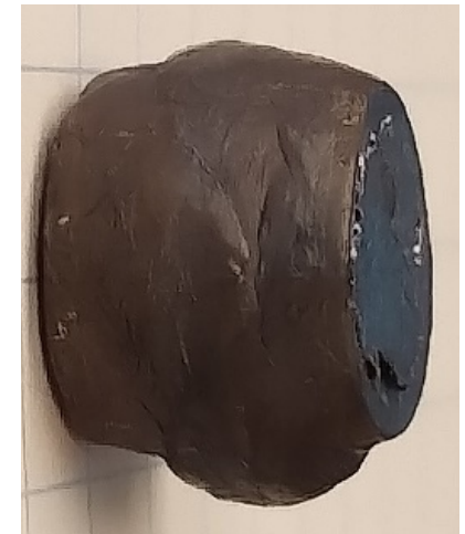
Non-uniform deformation in 70% height reduction sample
