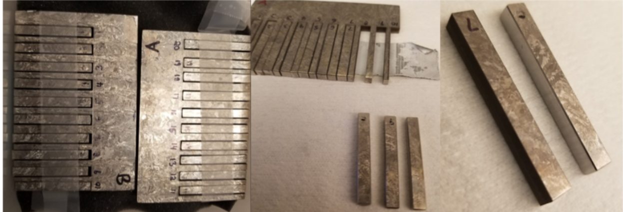
Fig. 9 Conventional fatigue beams sectioned via EDM, chamfered, polished and etched.
