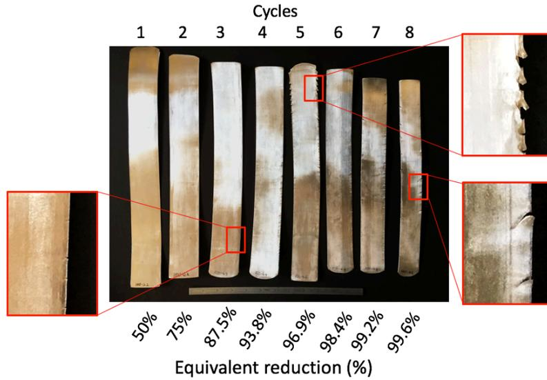
Figure 31.1: Samples of Al 1100 processed between one and eight successive roll bonding cycles. Equivalent rolling reductions are noted. Inset figures highlight edge cracks that form despite shearing between roll bonding cycles. Starting samples were about 50 mm wide.
