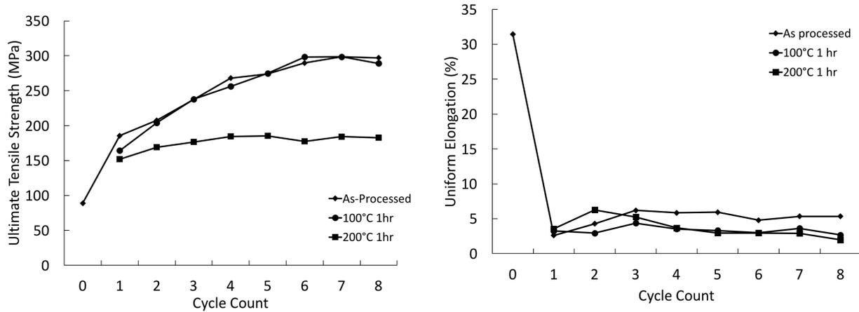
Figure 31.3: Strength (left) and elongation values (right) of roll-bonded material subject to heat treatments at either 100°C or 200°C for one hour.
