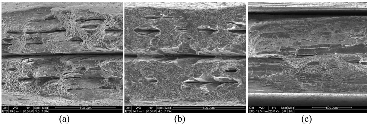
Figure 31.4: Tensile test fracture surfaces of Al 1100 subject to 5 cycles in the (a) as-processed (b) 100°C for 1 hour and (c) 200°C for 1 hour conditions. All samples were tensile tested at room temperature with a strain rate of  $1.6 \times 10^{-3} \text{ s}^{-1}$ .
