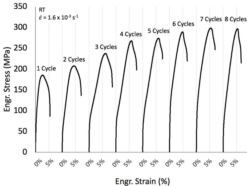
Figure 31.2: Stress-strain curves for as-processed samples subjected to one to eight ARB cycles.
