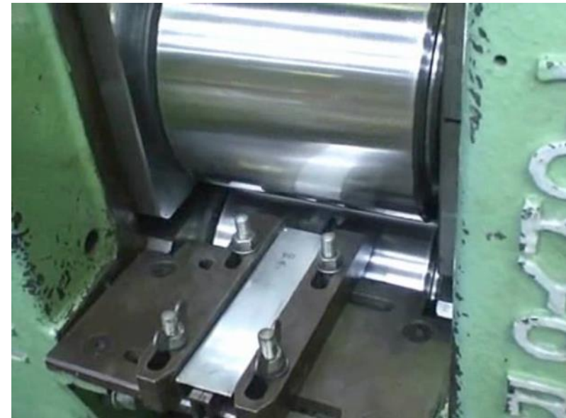
Fig. 15. Edge guides used on rolling mill for ARB studies at Osaka University [8].
