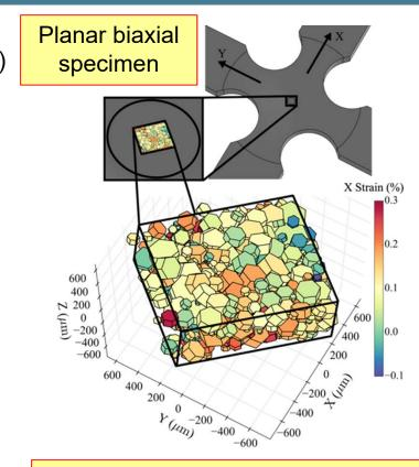
3D grain reconstruction from in-situ diffraction study
